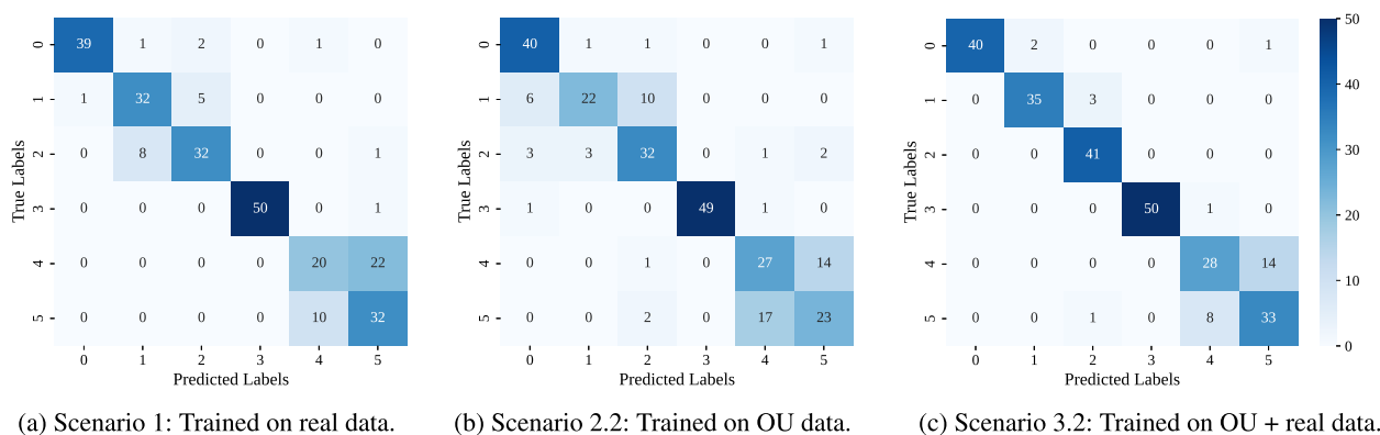
FIGURE 11. Confusion matrices illustrating model performance on predicting the target workstation 4 seconds in advance on the real-world dataset across different training scenarios: (a) Training on real data; (b) Training on Ornstein-Uhlenbeck (OU)-based synthetic data; (c) Training on OU-based synthetic data, then using transfer learning to further train it on on real-world data.
