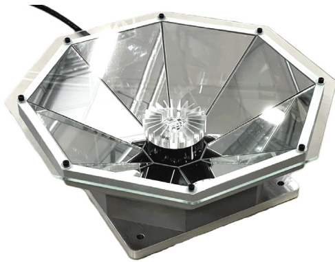
FIGURE 5. The LiDAR system reflects the entire FOV of the rotating LiDAR towards the scene, expanding the field of view, while maintaining the range and robustness of the rotating LiDAR. (© Atle Aalerud, 2024. Picture may be reproduced with attribution.)
